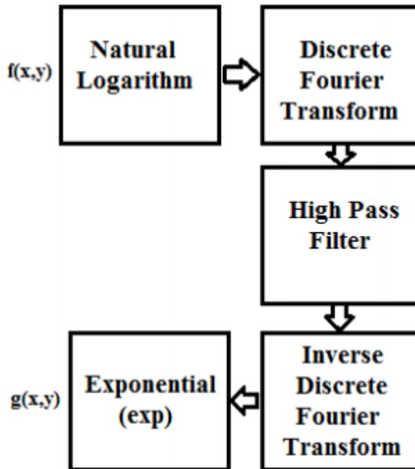
Figure 2: shows flow chart of homomorphic filtering
