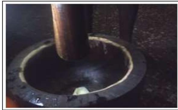
**Figure 1. Yam pounding mortar and pestle**
